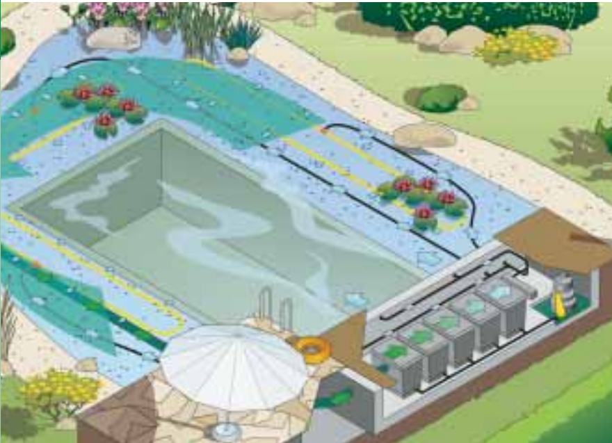
Schematic diagram: ProfiClear module filters are outstandingly suited for use on swim ponds
