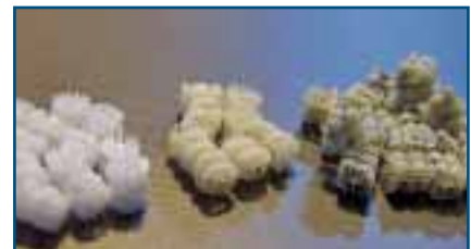
Biological surface for settlement of the microorganisms (left – biomedium that has not yet been used, right – with settled microorganisms).
